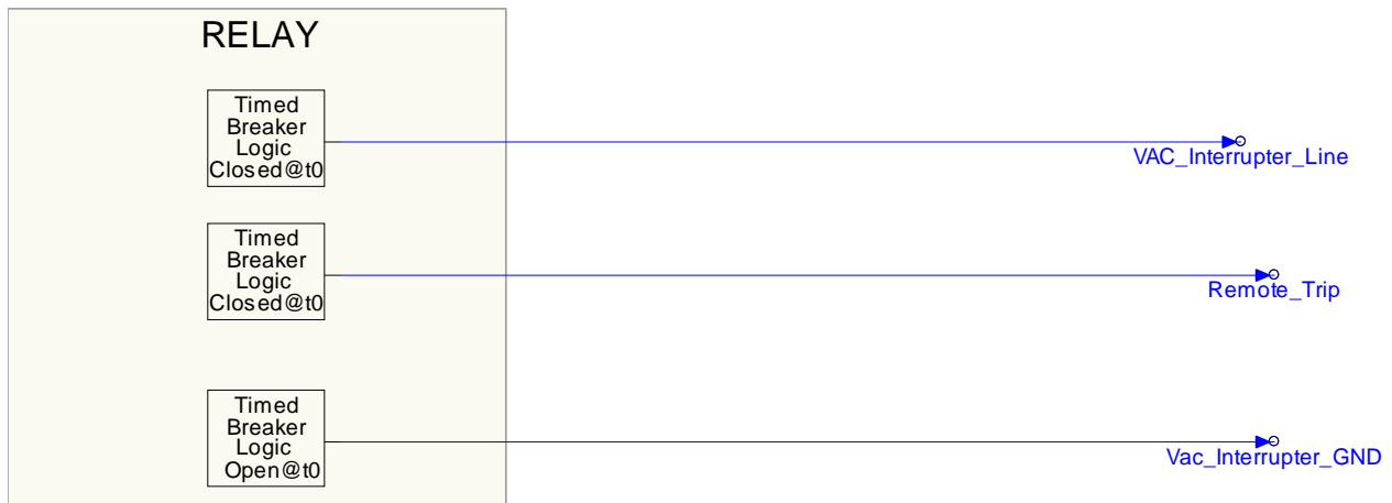
Figure 12. PSCAD Setup to Control the Breakers.
